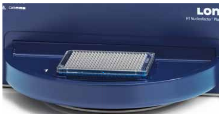
Figure 3.1: 384-well Nucleocuvette™ plate handler work area
