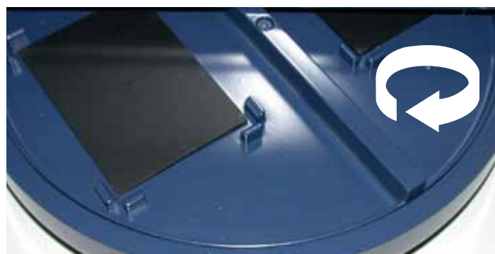
Figure 4.3: Turn carousel manually to recover samples
