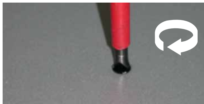
Figure 4.2: Lift contact bridge by turning the screw clockwise
